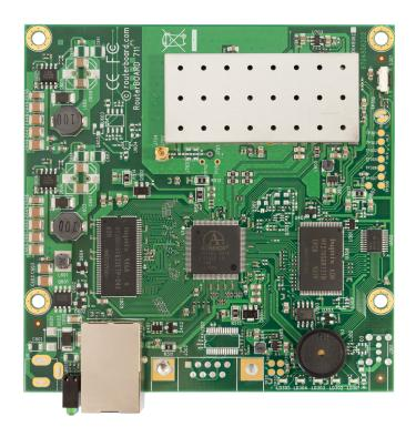
The RB711 is a small CPE type RouterBOARD wireless router with an integrated 5GHz 802.11a/n wireless card.
